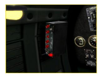
Touch flood light switches to toggle lights on or off.
